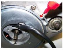
**Without** the new rotor in place, put the new stator base (the plate with the coils) onto the engine, so that the screwholes in the crankcase are about middle of the long holes.
