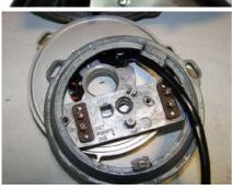
Put the stock (original) magneto holder plate now liberated of the old coils onto the backside (the one without the coils) of the new stator plate. In most cases both should stick to each other. Make sure that the long holes for the fastening screws match.
