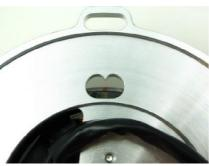
The newer version of this system offers some simplified way of setting timing. Here you have some window with a small pointer that should align with the marking on the rotor.
