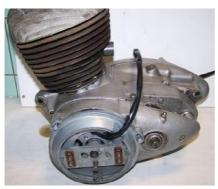
Place the whole assembly onto the engine - screws in middle of long holes and tighten the 3 screws.
