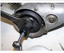
To disangage the new rotor again, use the puller which is supplied. It screws onto the hub of the rotor.
