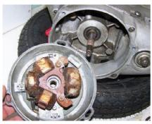
Disconnect all wires from the Wipac magneto and the silicone rectifier (so there was) and remove these parts.
