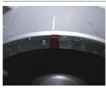
Have a look at the new rotor. You will find on its circumference a small line. That is an ignition marking. As it will not be visible once the rotor is in place, transpose it to the top of the drum wall (marker pen).
