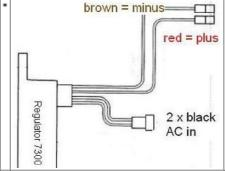
The new regulator/rectifier has 4 wires
